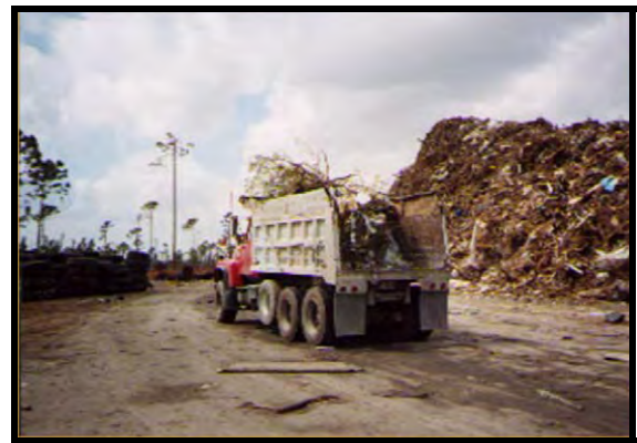
Figure 11.6 – Truck With No Solid Tailgate
