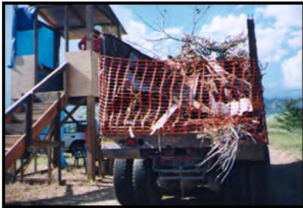
Figure 11.5 – Truck With No Tailgate
