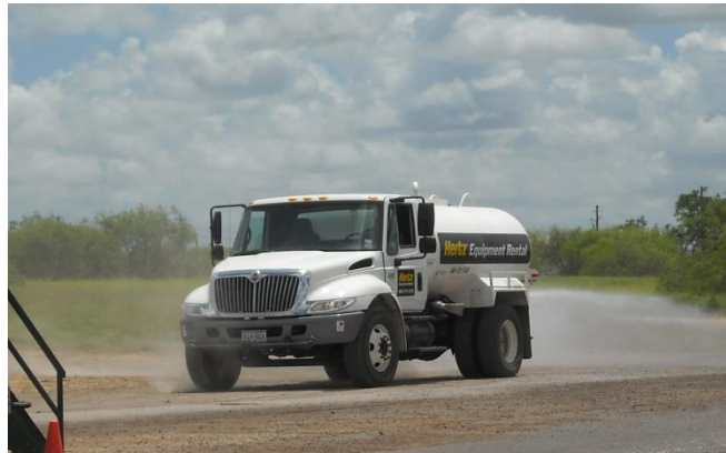
A water truck sprinkling to control dust on an access road.
